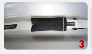
Insert the sensor as far as possible into the pocket.
