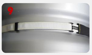
Slide the plastic eyelet ½ inch over the end of the strap. The sensor positon has no influence to the accuracy of the function, but it should not be directly positioned over a valve or valve hole (the sensor should have full contact with the rim).
