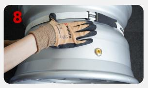
Make sure that the end of the strap is thoroughly pressed down and secured. To increase the pressure and improve the connection a round tool or the end of a screwdriver can be used.
