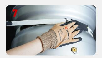
Close the hook and loop (velcro) fastener, make sure the upper and lower strap is properly aligned.
